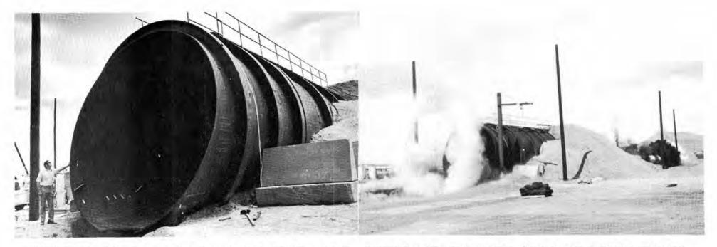
TEST SECTION of Sandia's new shock tunnel is checked by Manuel Vigil (9322), project engineer for the facility. The end of the 19-foot-diameter section is cut at a 75 degree angle to accommodate large test items which are
